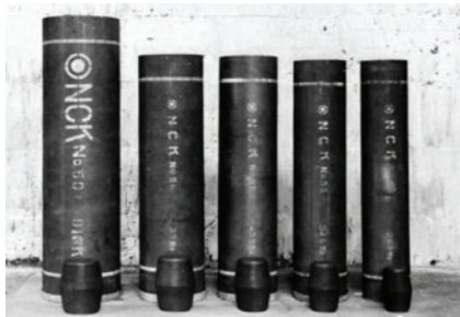
1927 Successful manufacturing of artificial graphite electrodes Successful manufacturing of Japan's first 6-inch to 12-inch artificial graphite electrodes
